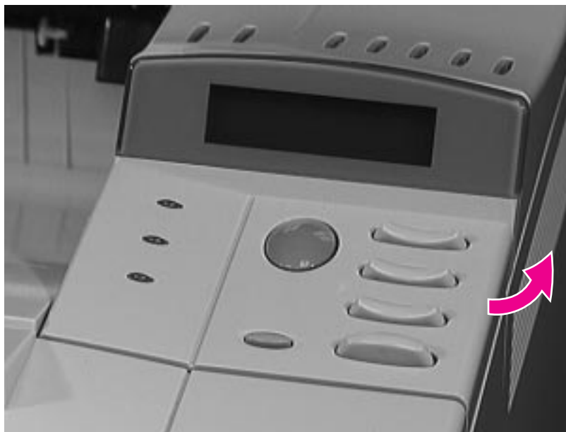
Figure 6-3 Removing the Control Panel Overlay
